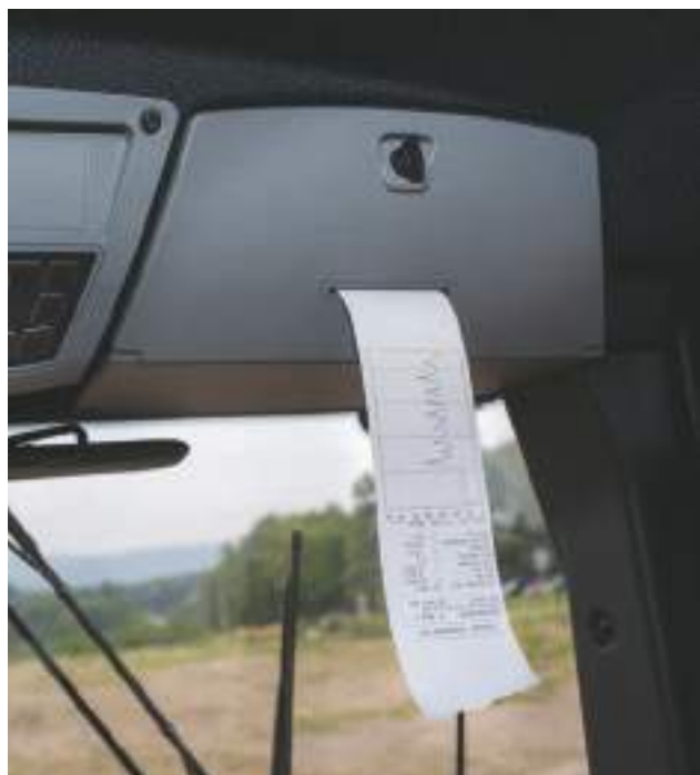
Integrated printer: for documentation of compaction results.
