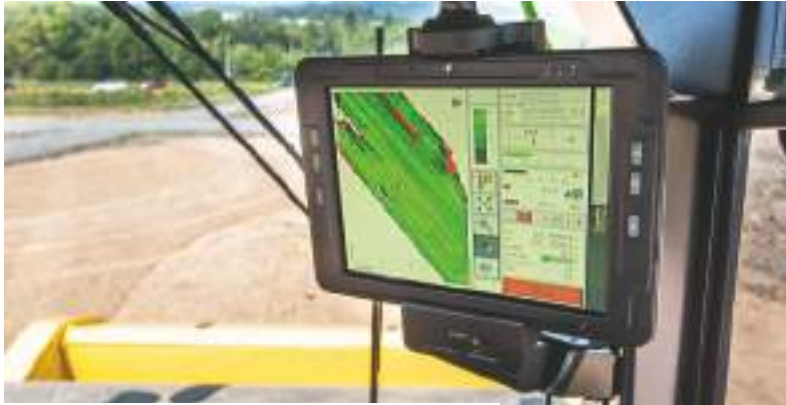
In colour: illustrated compaction maps including compaction results.
